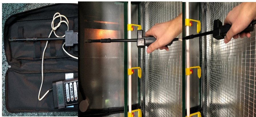
Fig. 4. Method for determining the air velocity in the technological module using TKA-PKM thermohygrometer-anemometer
